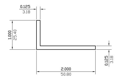
0.125(3.18)WALL THICKNESS EXCEPT AS SHOWN DATE REV DESCRIPTION BY 03/20/23 REMOVED ALLOY NDZAL 231.856 мм.2 IN.<sup>2</sup> 0.359 EST.AREA EST.AREA 0.424 0.631 EST.WT. LBS/FT. EST.WT. KG/M. 6.000 152.400 EST.PER. EST.PER. MM. OUT PER. MM. OUT PER. 2.236 56.796 C.C.D. C.C.D. FACTOR 14 **FINISH** M/F ALLOY & TEMP. 1:1 DWN BY C.P. SCALE DATE 08/18/2000 CKD BY
